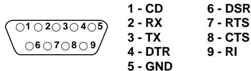
Figure 3-1. EIA 232 Service Port Pin Assignments
